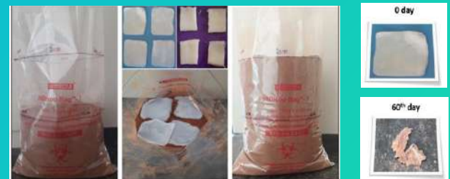
Bio-degradability tests in landfill
